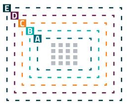
> RINGS A / C ensure fundamental electrical + functional compatibility between any CF3® module family with simple signal routing.
