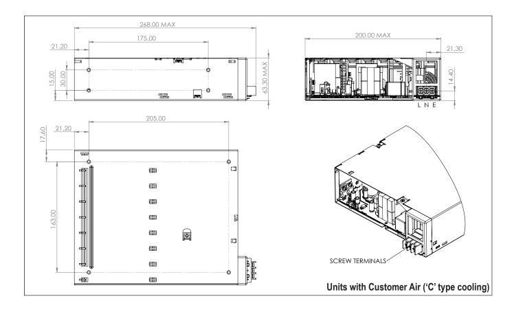
Customer fixings. 8 holes M4. Max thread penetration:- 4.5mm
