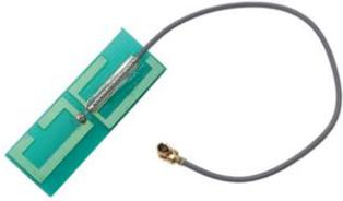
Laird Connectivity's Mini NanoBlade is a dual-band, vertically-polarized omnidirectional antenna designed to provide the durability and performance of the NanoBlade in a smaller form factor. The Mini NanoBlade has a gain of 2-2.5 dBi at 2.4-2.5 GHz and 2.5-4.8 dBi at 4.9-5.875 GHz.
