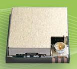
EMB-LR1276S is the new ultra low power LoRaWAN based wireless OEM Embit module. The EMB-LR1276S with its 11,5mm x 11,5mm form factor is the smallest LoRaWAN radio module available on the market. It embeds a full LoRaWAN™ Class A and Class C protocols and it enables to connect it to any LoraWAN™ compliant network infrastructure. Also, Semtech's proprietary spread spectrum modulation technique provides high inteference immunity.
